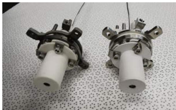
AM cathode (left) vs. traditionally manufactured cathode (right)
