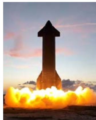
Starship SN24 fire test with two Raptor engines (court. SpaceX)
