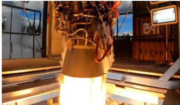
Fire test of the Helix engine in July 2022 (courtesy. RFA)
