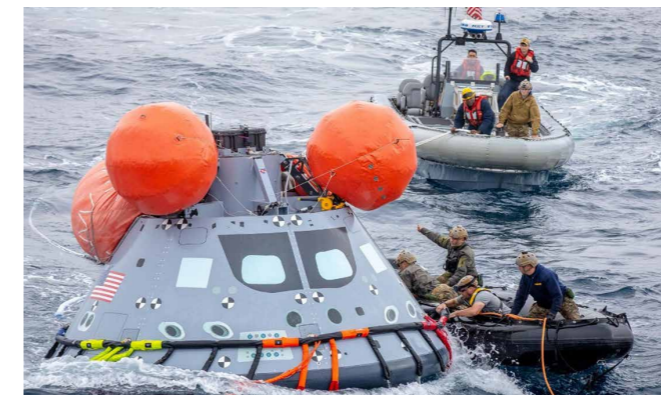
U.S. Navy divers from Explosive Ordnance Disposal (EOD) Expeditionary Support Unit 1, attach tending lines to a mock Orion capsule during Day 2 of Underway Recovery Test 9 (URT-9) aboard the USS John P. Murtha. During the weeklong test, NASA's Landing and Recovery team completed their final mission certification ahead of Artemis I.
