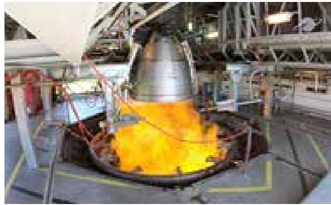
Test of the Vulcain 2.1 engine (cour. ESA)
